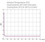
In operation state temperature is -86°C, Put in 48x1.8ml test tube (water filled) in freezer and the sample temperature reaches -86°C within 2.5min
