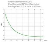
Put in 48\*1.8ml test tube (water filled), turn on the power and temperature reaches - 86°C within 120min
